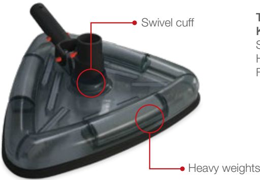
Transparent Triangular Vacuum Head K052CB/PRE Swivel cuff avoids entanglement of hose. Heavy plastic-coated steel weights. Fits 32 / 38mm (1¼ / 1½in) vacuum hose.
